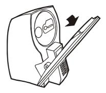
4.) Place a CD on the center spindle with the printed label side facing up. Press down near the center hole of the CD to make sure it is properly seated on the spindle.
